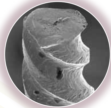
Micro-Cracks on Separated Instrument
